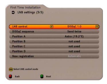
Select the required setting for your LNB control using the buttons (only on connection of the receiver to a satellite reception system). The following options are available:
